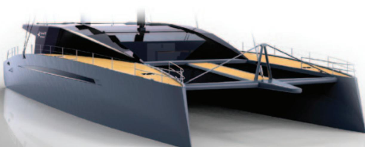
The Sunreef 80 Ultimate carbon fibre yacht has thin and sleek marine hulls with reversed bow and integrated stepped hull chins which is essential for the yacht's high performance. The superstructure will be shorter and more minimalist than on a conventional leisure catamaran which will add to the boat's lightness and streamlined look. The flybridge is an option here as the height of the boat decides on the level of air resistance.
