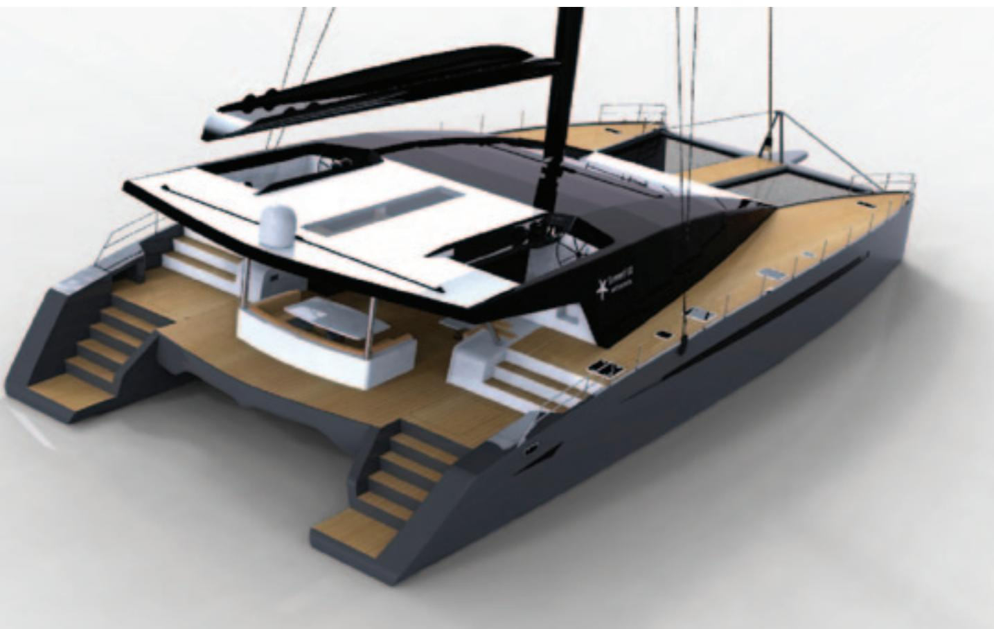
Two external helm stations will be placed on each side of the cockpit and a third one inside. The cockpit will feature the usual comfortable seating and dining area for 12 as well as a storage for water toys or the provisioning for long crossings.
