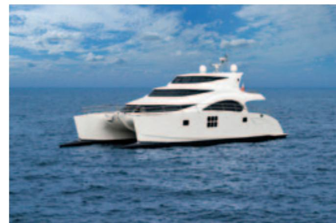
The exterior shape of the ONDIN features streamlined marine hulls meticulously designed by Sunreef's design studio with the help of Laurent Bourgnon to be as wave piercing as possible as well as underwater bulbs and aft platforms increasing the hull's length and enhancing the yacht's performance in natural way. The gigantic flybridge has undergone major changes and has been
